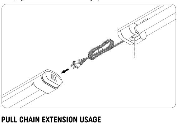
If the ceiling is too high, connect the extension chain to the pull chain end before completing installation.
