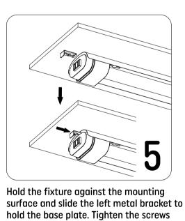
as needed to secure the fixture firmly in place.
