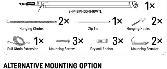
Use toggle bolt (not included) to replace drywall anchor, hanging hook and screw if needed.
