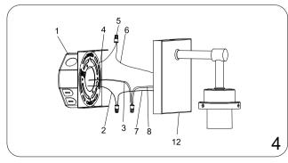
5. Attach fixture canopy[12] onto mounting bracket[2] using canopy nuts[10] previously removed in step 2. Tighten to secure fixture to the wall. Note: Fixture can be mounted in the up or down position.
