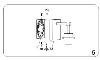
Screw recommended bulb[13] into socket. Align holes on the fixture metal body
