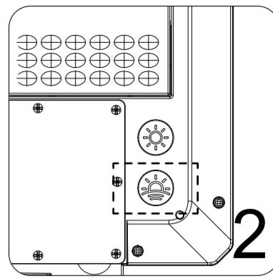
Set preferred color temperature. Press the CCT button to change the color temperature. The default setting is 6500K. Continue pressing button to select 5000K-4000K-3000K-2700K, then back to 6500K. Select from these white tone settings: 100%/50%/25%/Off
