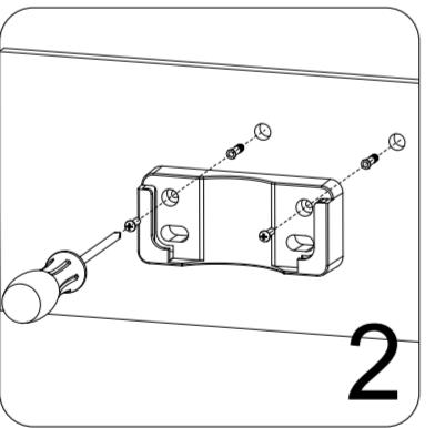
Note: Installation requires a 6-inch flat mounting surface unobstructed by trim or pipes as you will need to slide the fixture onto the bracket as the final installation step.
