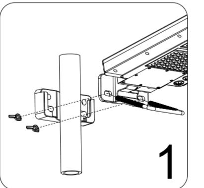
Place the mounting bracket on the pole. Align the holes on the solar street light to the oval holes of the mounting bracket. While gripping the street light and mounting bracket together, slide the U-bolt through the bottom oval holes as shown in the diagram. Use the wing nuts to securely tighten the solar street light to the bracket. Note: You may need help from another person for this step. Mount the fixture on 1.5" to 3" diameter poles.
