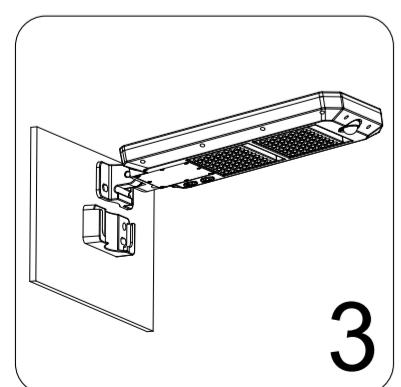
Align the street light with the mounting bracket and slide from the top to secure the street light to the bracket.
