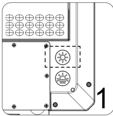
Press the On/Off button to test the fixture. It will light up for about 4 seconds.
