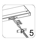
Gently pull the three quick connectors from inside the fixture. Using wire strippers, expose 3/8"-7/16" of bare metal on each supply wire. Insert the supply wires into the corresponding quick connector: Black to Black White to White Green to Green
