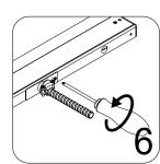
Gently push the wires back inside of the fixture. Secure the connection cover back onto the fixture assembly.
