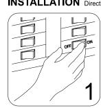
Turn off power source to the power supply you are installing the fixture on.
