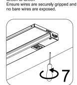
Place the fixture in the desired position. Mount the fixture using a Phillips-head screwdriver, fully seating the pre-installed mounting screws. Provided screws are suitable for cabinet bottoms 3/8" or thicker. It may be required to pre-drill a pilot hole for the screws using a 3mm or 1/8th inch size drill bit if needed.
