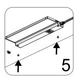
Push in the screw hole covers, covering the two exposed screws. When not linking fixtures, push the end caps in the OUTPUT port.
