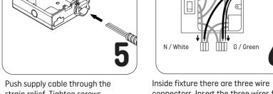
connectors. Insert the three wires from the supply cable into the corresponding wire connectors as shown above. Make sure that all wires are securely gripped, and no bare wires are exposed.
