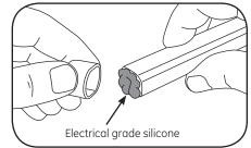
At any open end, apply electrical grade silicone and press fit a light guide end cap to the Tetra Contour.
