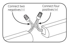
6 Use twist-on wire connectors to join wires together. Fold wires behind light engines.
