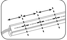
2 If required, cut wire loops between sections or through light engine (refer to the Cutting Resolution Chart above).
