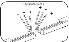
Separate wires and identify outer conductors as positive (+) and middle conductors as negative (-). Strip ends back 0.5 in. (13mm).
