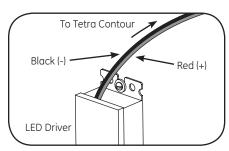
Run supply wire from the LED Driver to a section of Tetra Contour.
