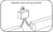
Insert wire connectors into weather box. Fill with electrical grade silicone and close box. Weather box can be mounted using #8 (M3) screws.
