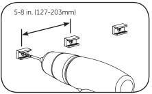
1 Install a light engine mounting clip, using #6 (M2) counter sink screws, every 5–8 inches (127–203mm) on center until the end of the run is reached.
