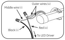
3 Connect the two outer wires (+) from the LED strip to the red wire (+) of the LED Driver. Connect the middle wire (-) from the LED strip to the black wire (-) of the LED Driver.
