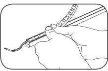
**3** Push the light engine segments down into the light quide.
