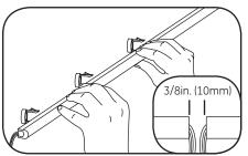
Attach Tetra Contour to the mounting clips, leaving a 3/8 in. (10mm) gap between sections to allow for expansion or contraction. For additional security, twist neon tie-wire around mounting clip and light guide.
