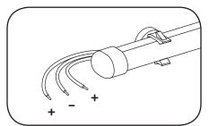
Separate wires and identify outer conductors as positive (+) and middle conductor as negative (-). Strip ends back 0.5 in. (13mm).
