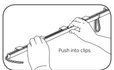
Push each 16 in. (406mm) light engine segment into the clips. Fold loose wires into the channel of the light engine mounting clips.
