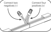
Use twist-on wire connectors to join cut wires together. Fold wires behind light engines.
