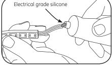
6 CAUTION: Anytime light engine or supply wire is cut and wire is exposed, electrical grade silicone must be applied (see list on the next page for recommendations).
