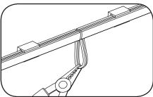
If required, cut wire loops between sections or through light engine in the appropriate area (refer to the Cutting Resolution table above).
