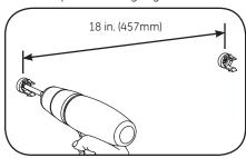
1 Install a minimum of one light guide mounting clip per 18 in. (457mm) using #10 (M4) screws.
